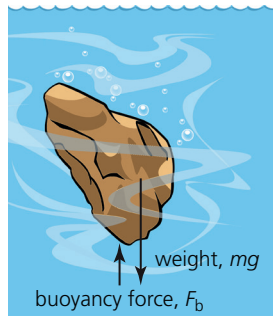
■ Figure A2.10 Forces on an object immersed in a fluid
